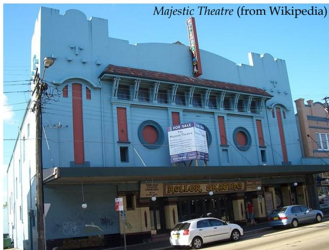
In 1979, to accommodate its use as the Majestic Roller Skating Rink, further alterations included the removal of the original sloping theatre floor and replacement with a concrete slab, destruction of the dress circle seating and replacement of timber windows and doors with aluminium. The building has been vacant for some years, and appears to be in poor repair. A number of developments have been approved by Council in recent times but none has proceeded.
